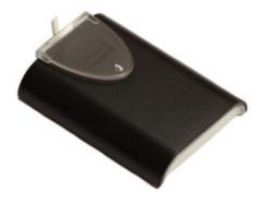
The 5427 CK from Omnikey is a USB contactless smartcard reader that supports both low and high frequency technologies, providing a useful integration path for environments using a mixed range of credentials. Conforming to ISO 14443 A/B, ISO 15693 as well as HID Prox, the second-generation Omnikey 5427 CK is a platform independent reader that functions in many different environments, thanks to its support for both CCID and keyboard emulation functionality.
